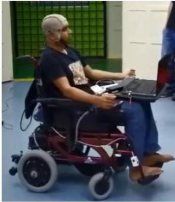
Fig. 2. BCIs using Electrooculogram for wheelchair navigation by ACRLAB, Universiti Malaya [6], [7].
