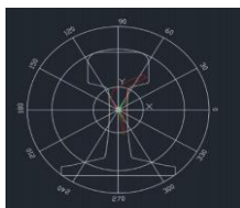
Fig.5 Polar coordinates for circumferential localization
