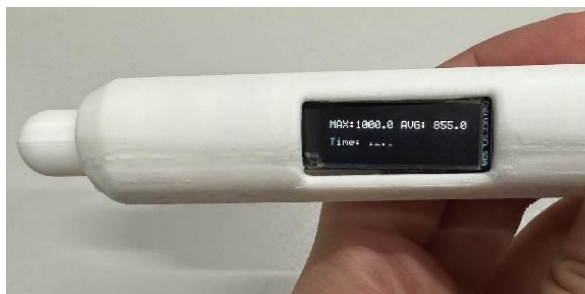
Fig.12 Pressure sensing massage stick test results
