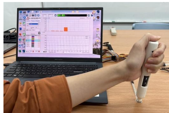
Fig.10 The left side shows the pressure value of the company's software, and the right side shows the 1kg force test of this design.
