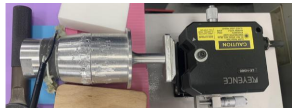
Fig. 2 Schematic diagram of transducer with amplitude horn
