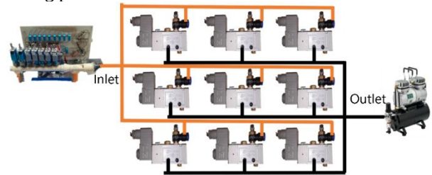
Fig. 3. The connection diagram of the third-generation tuning pneumatic valves
