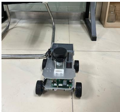
b. Mobile base with temperature and humidity ,wind speed detection module
