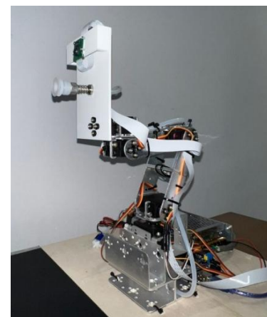
Fig. 5. Floor Tiling Robot Prototype.
