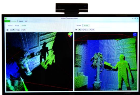
Fig.6 Kinect can create 3D imagery throughout the room and capture human body contours.
