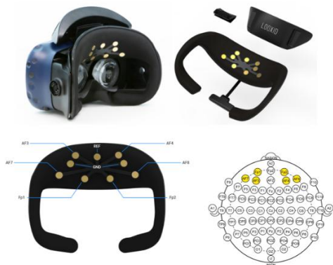
Fig. 6. HTC VIVE Pro HMD, a face gasket with the EEG sensors (top) and Looxid Link EEG electrode placements(bottom).
