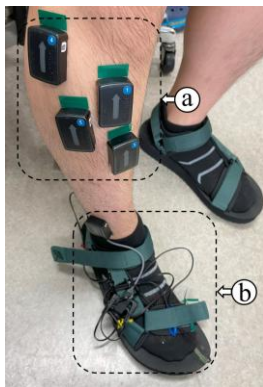
Fig.3. Sensor arrangement for data acquisition; a) wireless sEMG sensor assembly, b) wireless FSR sensor attachment
