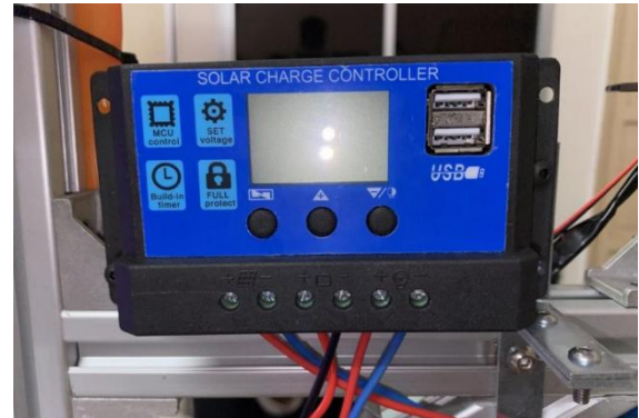
Fig. 5. Solar charge controller.
