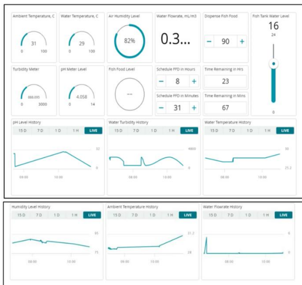
Fig. 7. System performance monitoring on the Arduino IoT cloud web dashboard
