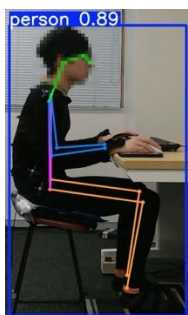
Fig. 5 Example of Poor Representation of Posture Features by YOLO Pose Estimation Results.
