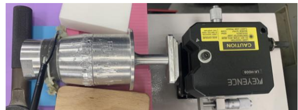
Fig. 2 Schematic diagram of transducer with amplitude horn
