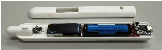
Fig. 7 pressure sensing massage stick internal Electronic Components
