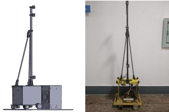
Fig.1 Exterior and physical view of the inspection robot
