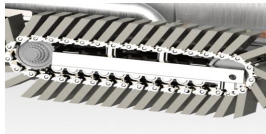
Fig.1 The design of the amphibious wheel
