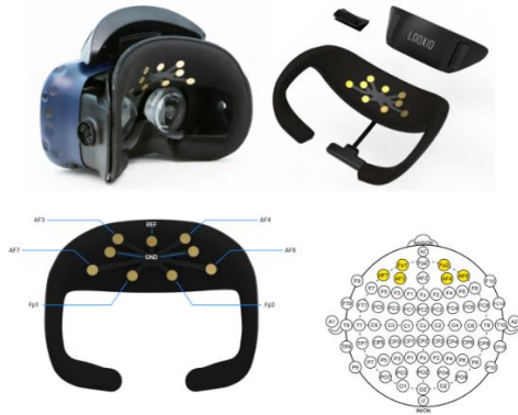
Fig. 6. HTC VIVE Pro HMD, a face gasket with the EEG sensors (top) and Looxid Link EEG electrode placements(bottom).
