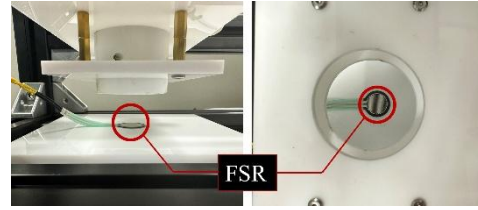
Fig 2. Force measurement instrument utilizing a force sensing register.
