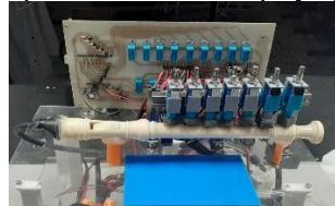
Fig. 2. Reciprocating electromagnet pressing system
