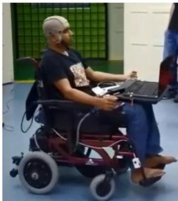
Fig. 2. BCIs using Electroocoulogram for wheelchair navigation by ACRLAB, Universiti Malaya [6], [7].
