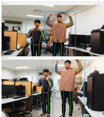
Fig. 3. Multi-Person and detected keypoints in 2D for applications of skeleton overlays.
