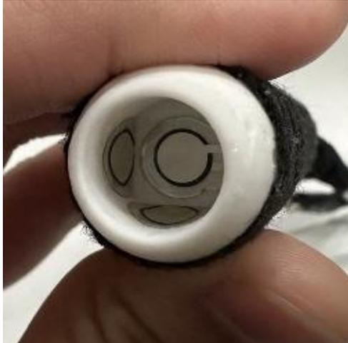
Fig. 1 Single Point Pressure Sensor
