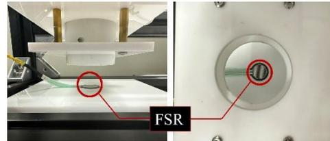
Fig 2. Force measurement instrument utilizing a force sensing register.
