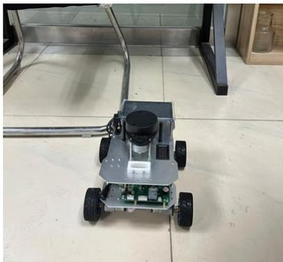
b. Mobile base with temperature and humidity, wind speed detection module
