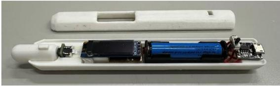
Fig. 7 pressure sensing massage stick internal Electronic Components
