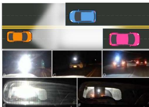
Fig. 4. Prototype and Control Process of Programmable Headlights
