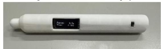
Fig. 6 pressure sensing massage stick final design of the physical appearance
