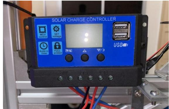
Fig. 5. Solar charge controller.
