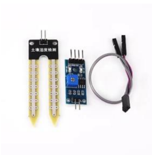
Fig. 5 LM393 Soil moisture sensors
