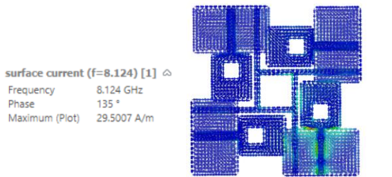
Fig. 7 Surface current distribution of four-port UWB MIMO antenna at resonant frequency, 8.124GHz.
