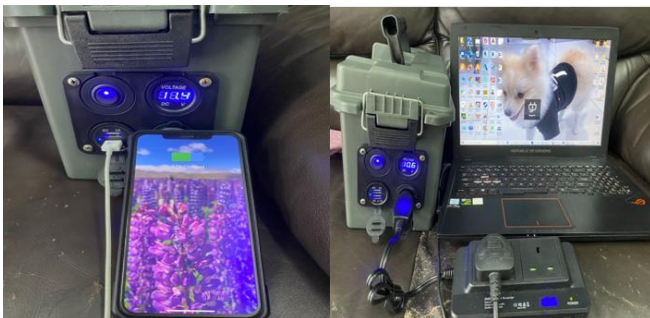
Fig. 4 The charging mobile phone and laptop with using the charging station
