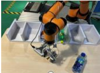
Fig. 11 Robotic arm grabs shaft hole
