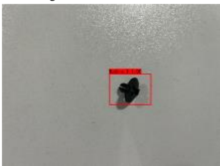
Fig. 8 Shaft hole image after inspection by YoloV4
