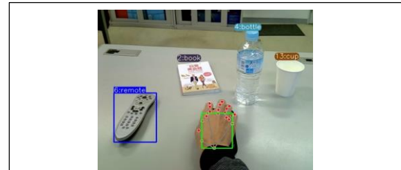
Fig. 1 Object detection results. (The target object is drawn in a blue bounding box and the user's hand is in a green box.)
