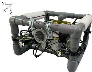
Fig. 2 View of developed low-cost underwater robot
