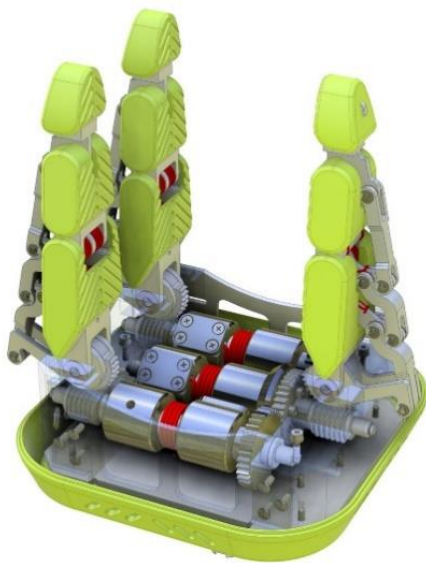
Fig. 3. The constructed anthropomorphic gripper with three executive groups of links.
