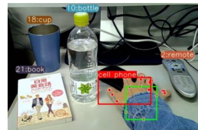
Fig. 2 Result of object location estimation (When the target object is estimated, it is surrounded by a red bounding box.)
