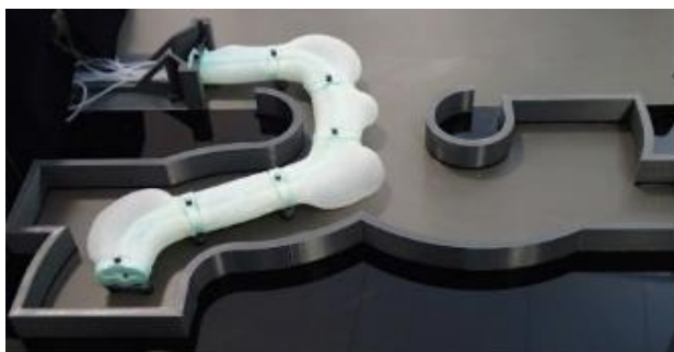
Fig.2 Pneumatic driven flexible manipulator [4]
