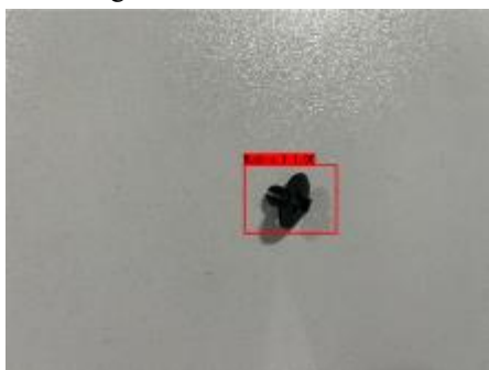
Fig. 8 Shaft hole image after inspection by YoloV4
