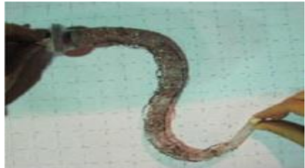
Fig.1 SMA flexible mechanical arm [3]
