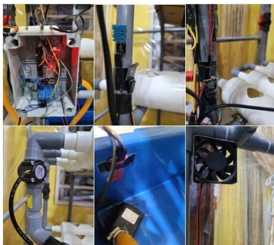
Fig. 11. Placement of Electrical Components
