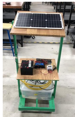
Fig. 1 Solar agriculture water pumping system prototype
