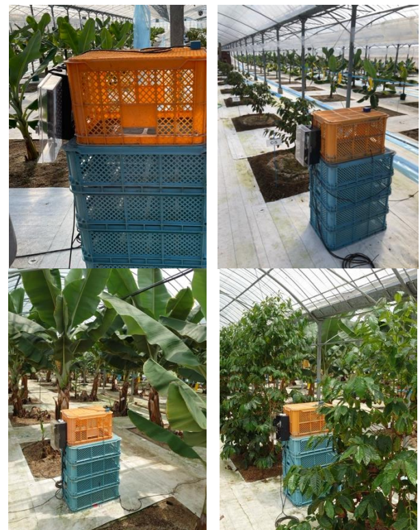
Fig. 5 Installation of the developed IoT modules (Right: coffee field, Left: banana field, Top: before growth, Bottom: after growth)
