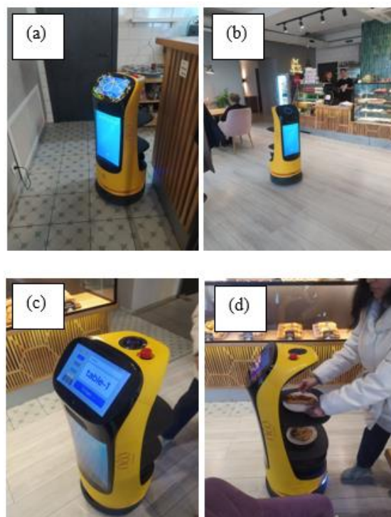
Fig. 2 Different phases of the robot work: (a) Robot waiting for collecting food items (b) Moving towards a destination table (c) Robot reached the destination table (d) A customer taking the food item from the robot
