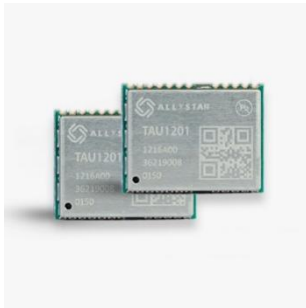
Fig. 9 Appearance of the TAU1201 module
