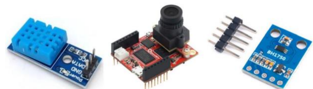
Fig. 5 The digital temperature and humidity sensor, light intensity sensor and OpenMV
