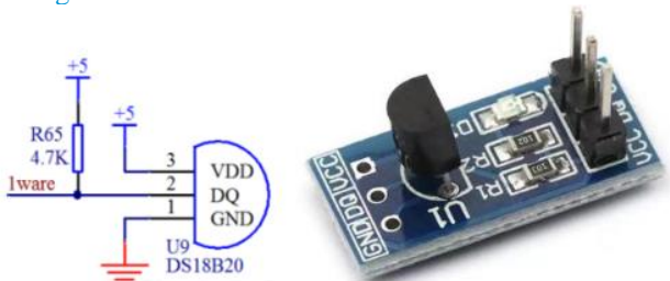
Fig.11 DS18B20 temperature sensor circuit schematic
