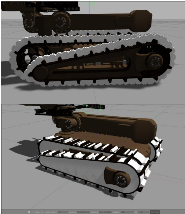
Fig.4. Track approximation with arrays of gear-wheels: small-sized (top) and large-sized wheels (bottom)[29]
