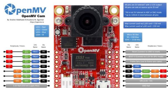
Fig.4 The pin definition for Openmv
