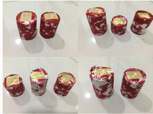
Fig. 1 Specimens fabricated under different heating temperatures and duration
