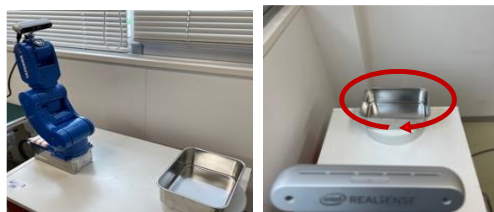
Figure 3. Experimental environment: (Left) A camera fixed on the robot and the metal tray on the rotating stand; (Right) a metal tray viewed from the camera; the metal tray is rotated clockwise and photographed.
