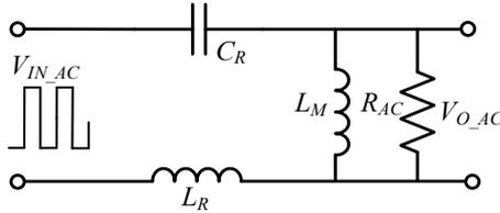
Fig 5 LLC series-parallel resonant tank equivalent circuit diagram
