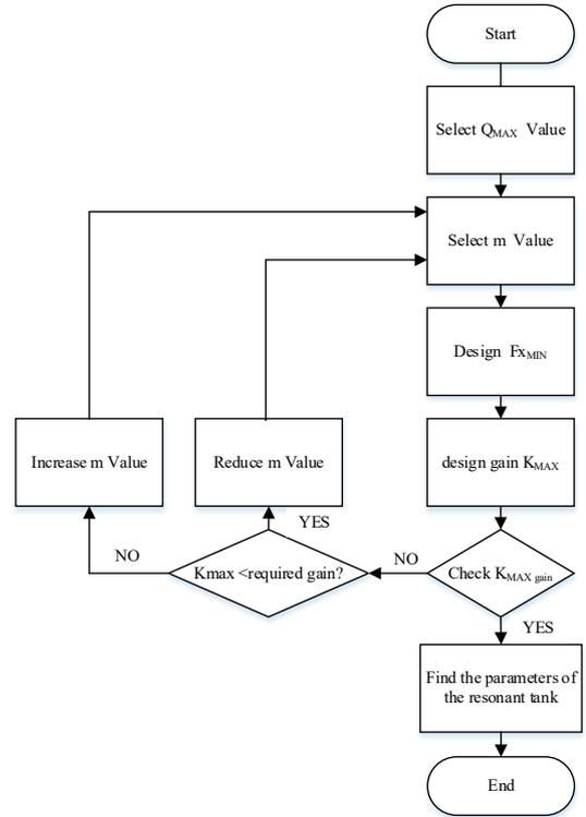
Fig 6 Resonant tank parameter design flow chart
