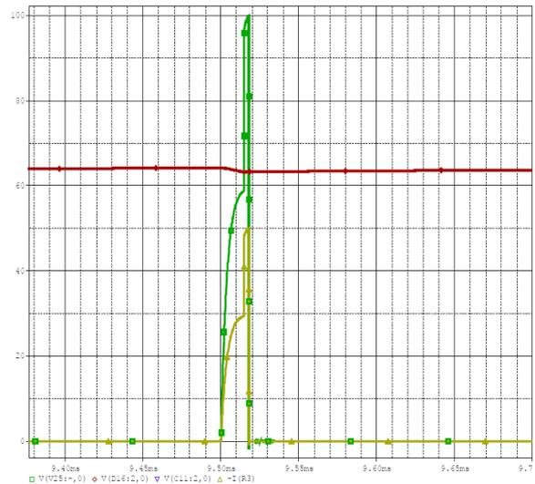
Fig 8 Results of parallel LLC simulation (green is output voltage; yellow is output current)
