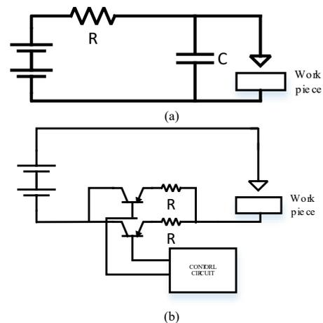
Fig 1(a) Resistance Capacitance (RC) power;
