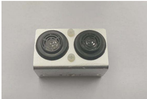
Fig.6. ULB-1 Ultrasonic ranging sensor
