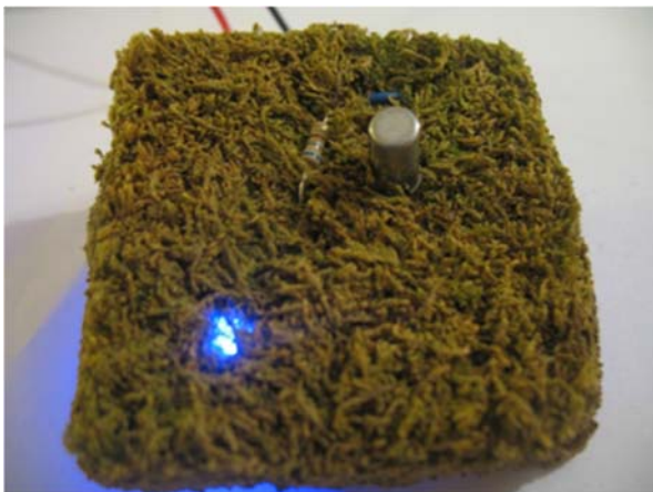
Fig. 4. A detail of a sense-and-actuate module to be mounted on PixelBeing' suit. Later prototype. A biomaterial-based circuit made out of natural wood and moss.
