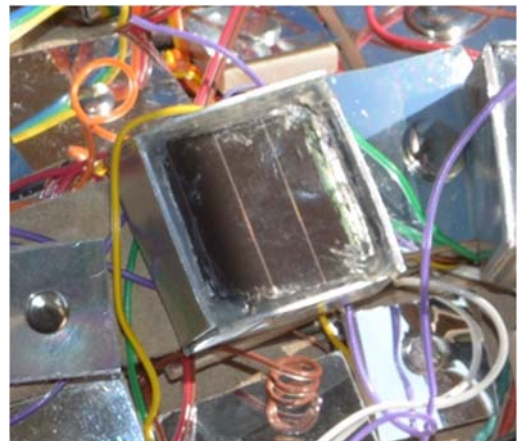
Fig. 3. Detail of the PixelBeing mask. A Solar-panels based circuit module mounted on PixelBeing's helmet
