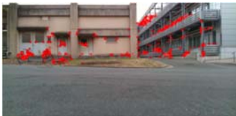
Fig. 1 Example of extracted feature points from ORB
