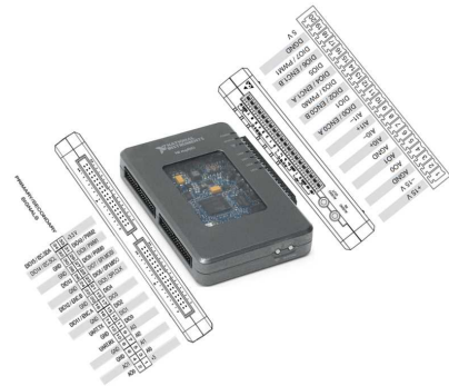
Fig. 2 MyRio-1900 control box
