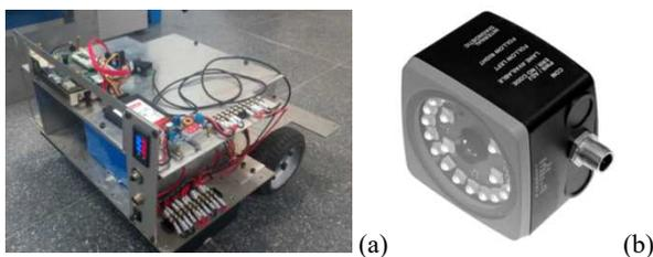
Fig. 1. (a) a differential wheeled robot platform equipped with an industrial PC (b) the optical reading head (PGV 100 serial) for barcode tag identification
