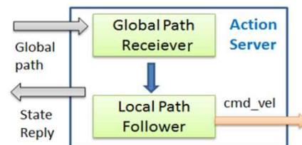
Fig. 5. An Action Server framework for AGV navigation
