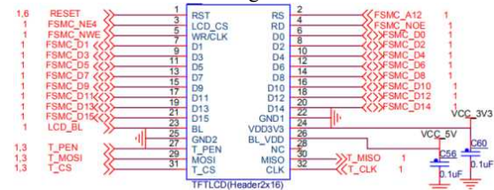
Fig.7. The hardware schematic of LCD9341
