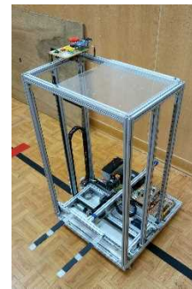
Fig. 4. Our experimental auto-stacking warehouse truck.
