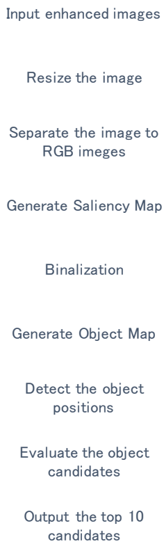
Fig.1 Flow of image processing
