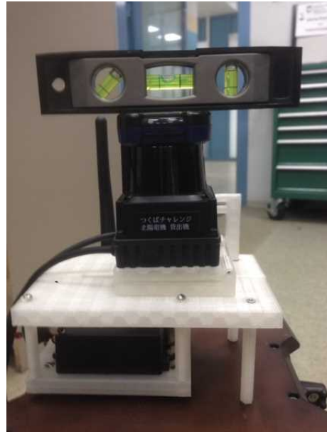
Fig. 2. Hokuyo laser on a stand. Laser is strictly parallel to the surface of the floor.
