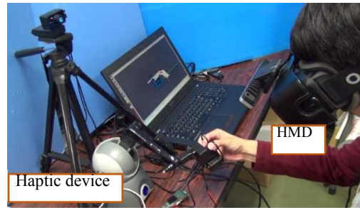
Fig. 2 Robot operation device with haptic device [4]
