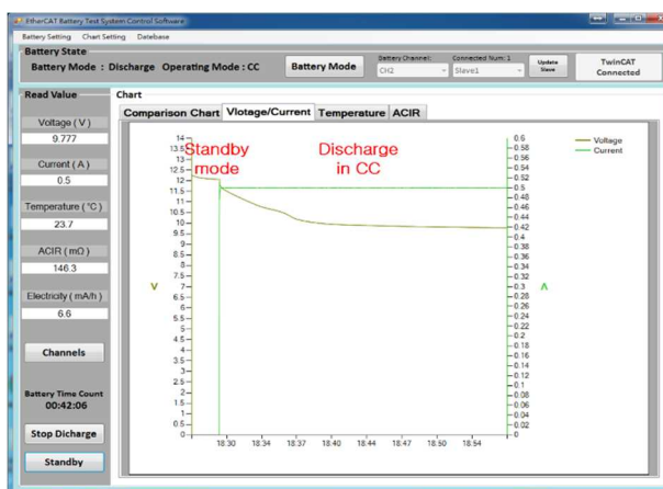
Fig. 7. Battery discharging in CC mode
