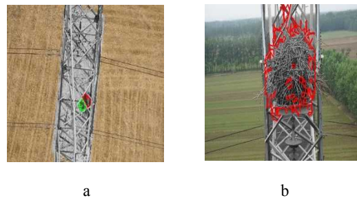
Fig. 6. The detection results of the bird's nest on the pylon under different backgrounds
