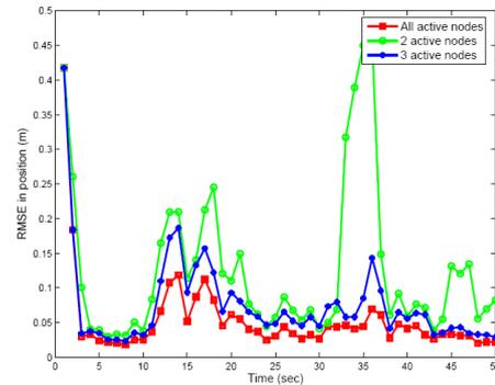
Fig.1 RMSE in position of the proposed filter.
