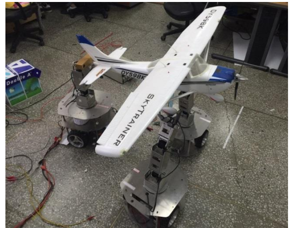
Fig. 4. Mobile Robots in formation based on the Vision.
