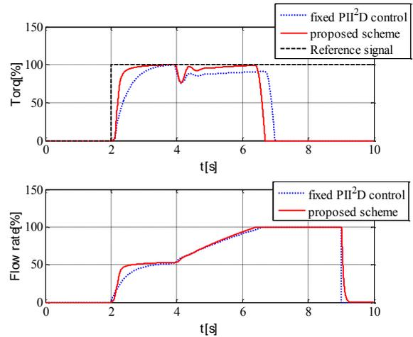
Fig. 3. Control results by fixed PII<sup>2</sup>D control and proposed scheme.
