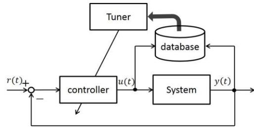
Fig. 2. Schematic of the data-driven control system.
