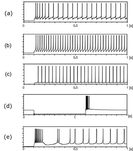
Fig. 4 Waveforms generated by the DSSN unit of RS (a), FS (b), LTS (c, d), IB (e). Excitable step inputs rise at  $t = 0.1$  (a-c,e). inhibitory step inputs are provided from  $t = 0.2$  to  $t = 1.0$  (d).
