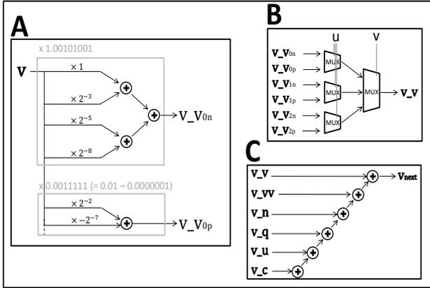
Fig. 1 Block diagram of the  $v$ -circuit. Symbols  $\times$ ,  $+$  and  $MUX$  mean a multiplier, adder, multiplexer, respectively. (A) Multiplication realized by shift operation and adder. (B) Add operation of the differential equation of  $v$ . (C) Correct  $v_{ij}$  are chosen by multiplexer depending on  $v$  and  $u$ .
