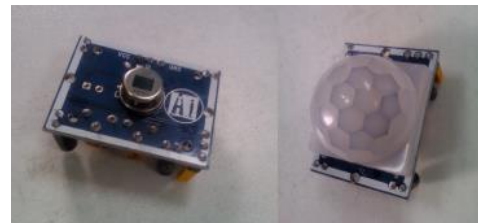
Fig 6. The sensors of infrared detector for human body
