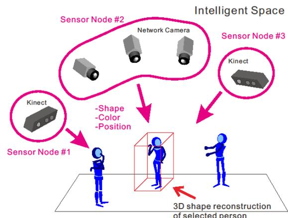
Fig 1. 3D shape reconstruction system
