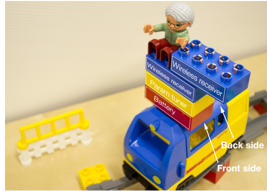
Fig. 6. Overview of the train system
