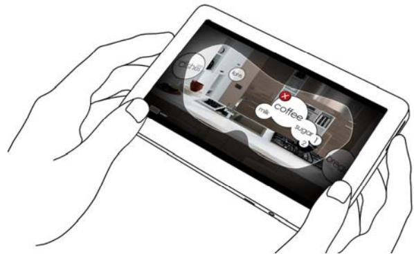
Fig. 1. Seeing through the eyes of the robot, including context depending action possibilities, varying in size depending on their likelihoods.
