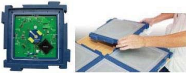
Figure 1: Left: The interior of the modular interactive tiles. Right: Assembling of a tile play field.
