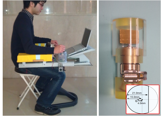
Fig. 2: Experimental system and vibration motors with eccentric mass on the shaft
