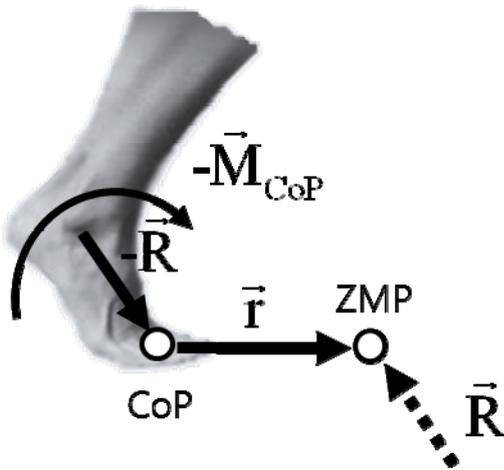
Fig. 2. ZMP, CoP and GRF. Adapted from [6].
