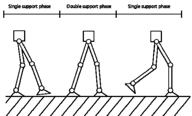
Fig. 1. Gait phases of the exoskeleton. Adapted from [5].
