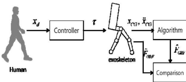
**Fig. 5.** Block diagram for proof of the algorithm
