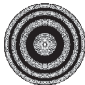
Fig.5: Low frequency moiré fringes from proposed target when \theta = 0, \beta = 0, h = 100mm
