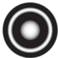
Fig.6: Low frequency moiré fringes from existing target when \theta = 0, \beta = 0, h = 100mm
