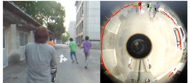
Fig. 7. Experiment of recognizing running people with the robot system in motion
