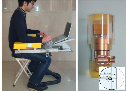
Fig. 2: Experimental system and vibration motors with eccentric mass on the shaft
