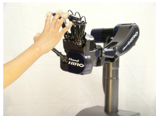
Fig. 3. HandHIRO, five-fingered haptic interface robot
