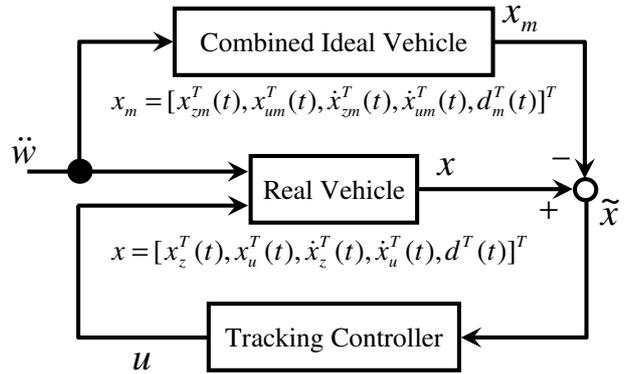
Fig. 2 Configuration of active suspension control system.
