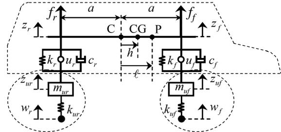
Fig. 1. Two wheels model.
