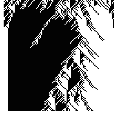
Figure 3: The spatio-temporal pattern which generated by PCA without the conservation of mass. The black cells indicate 1 and the white cells are 0. The vertical axis represents time step and the horizontal is space.
