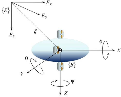
Fig. 1. Coordinate systems of AUUV
