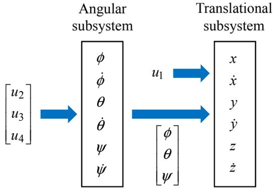
Fig. 2. Connections of rotational and translational subsystems
