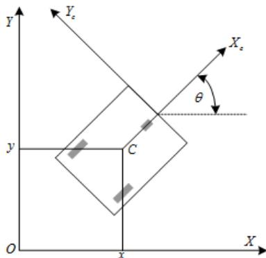
Fig.2. 2-D of a wheeled mobile
