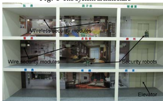
Fig. 2 The platform of the security system
