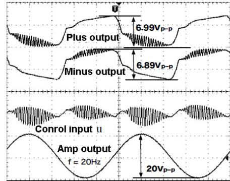
Fig. 11. Experimental results by PI control at  $C_0 = 220[\mu\text{F}]$
