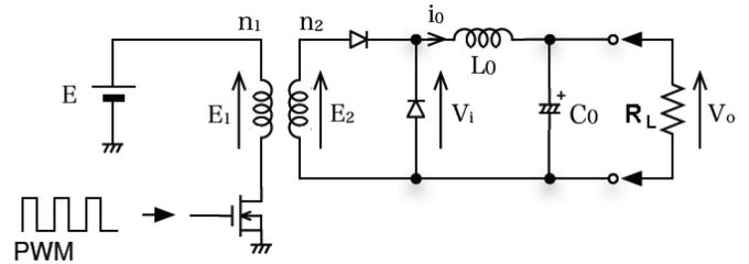
Fig. 2. Plus side model of power supply
