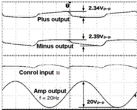
Fig. 8. Experimental results by the approximate 2DOF robust digital control at  $C_0 = 1000[\mu\text{F}]$
