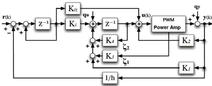
Fig. 7. Approximate 2DOF robust digital control system
