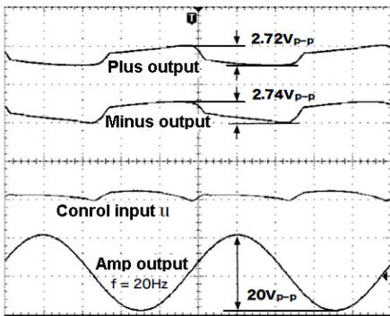
Fig. 9. Experimental results by the approximate 2DOF robust digital control at  $C_0 = 220[\mu\text{F}]$
