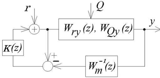
Fig. 6. System reconstituted with inverse system and filter
